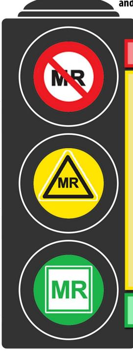
and other equipment used in or near the MR environment should be labeled as MR Unsafe, MR Conditional, or MR Safe.
